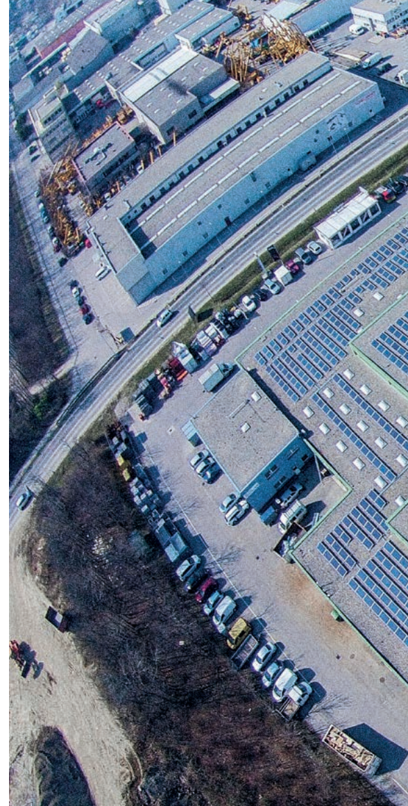
Electricity generation from the sun is an ideal supplement to wind energy: two photovoltaic systems with 350 kW, each in Brunn am Gebirge
